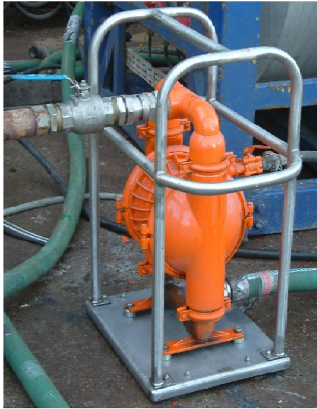
2" Air Driven Wilden & Sandpiper Chemical Pumps (ATEX Approved)
